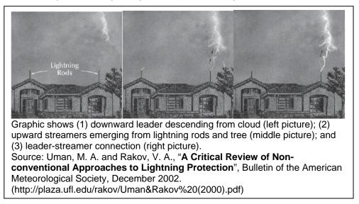
In the lightning attracting system, their inventors claimed that their air terminals can generate these upward streamers earlier than other natural objects on the ground can (hence the term "early streamer" was introduced in the early 1990s). To generate the upward streamers, the inventors initially used radioactive materials but these were replaced with other methods when the use of the radioactive materials was banned by governments worldwide.
