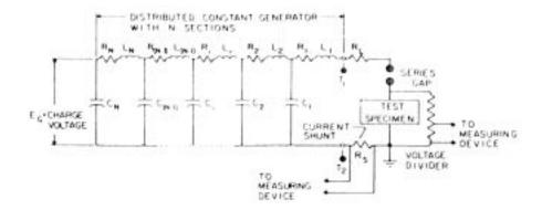
$R_A=$  ohms resistance  $R_L$  of leads from test specimen to terminals  $T_1$  and  $T_2,*R_S$   $R_S=$  ohms resistance of current shunt  $R_i=$  ohms section resistance  $C_i=\mu F$  section capacitance  $L_i=\mu H$  section inductance
