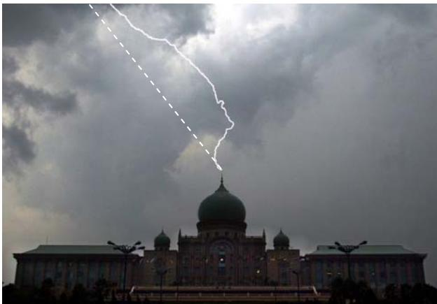
Fig. 9: The dotted line represents the hypothetical path of the early streamer according to the ESE hypothesis.
