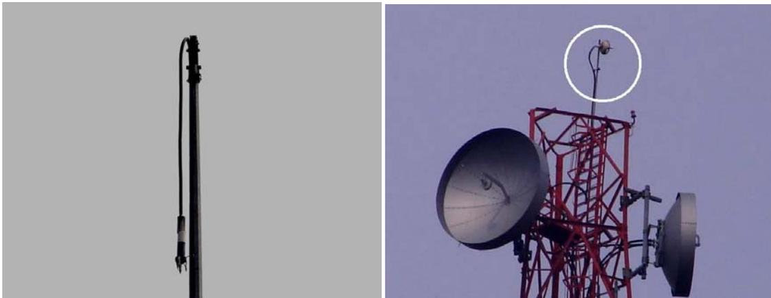
Fig. 13 – Photographs showing the ESE (left) and CVM (right) air terminals hanging by their down conductors as a result of damages to their non-metallic mounting poles.
