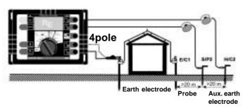
The standard earth test, usually called the 'Fall of Potential Method' uses either 3 or 4 poles or connections. The four pole method compensates for any voltage drop there may be in the wire used to connect to the earth E under test. The fourth wire is particularly important if the connection to the E is a long distance from the instrument.
