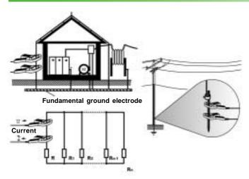
In this method the temporary stakes are replaced by two current clamps. The test current from the E and the H/C2 terminals of the instrument is fed through a current clamp. This clamp is placed aroung the conductor connecting the earth under test. A second measuring clamp is placed around the same conductor.
