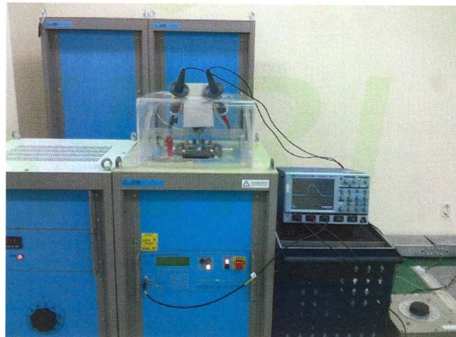
Photo. SG02 : Measurement of residual voltage test and operating duty test
