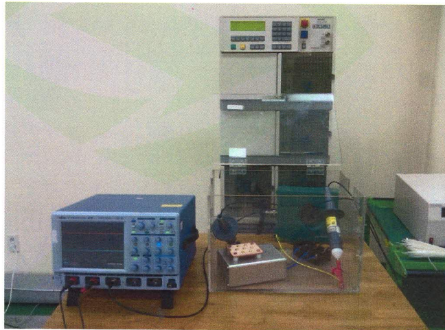
Photo. SG03 : Measurement of the front of wave sparkover voltage test
